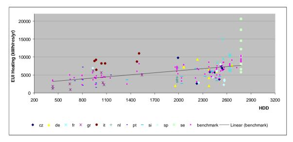
Figure 34: EUI4 (kWh heating /resident/yr) versus HDD
