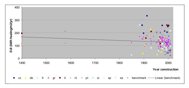
Figure 29: EUI3 (kWh heating /m2/yr) versus year construction
