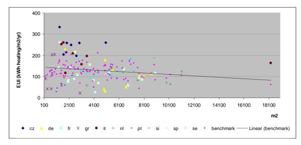
Figure 25: EUI3 (kWh heating /m2/yr) versus m2
