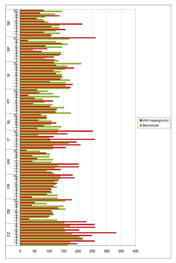
**Figure 24:** Real heating energy consumption per square meter, kWh heating/m2/yr, and the benchmark
