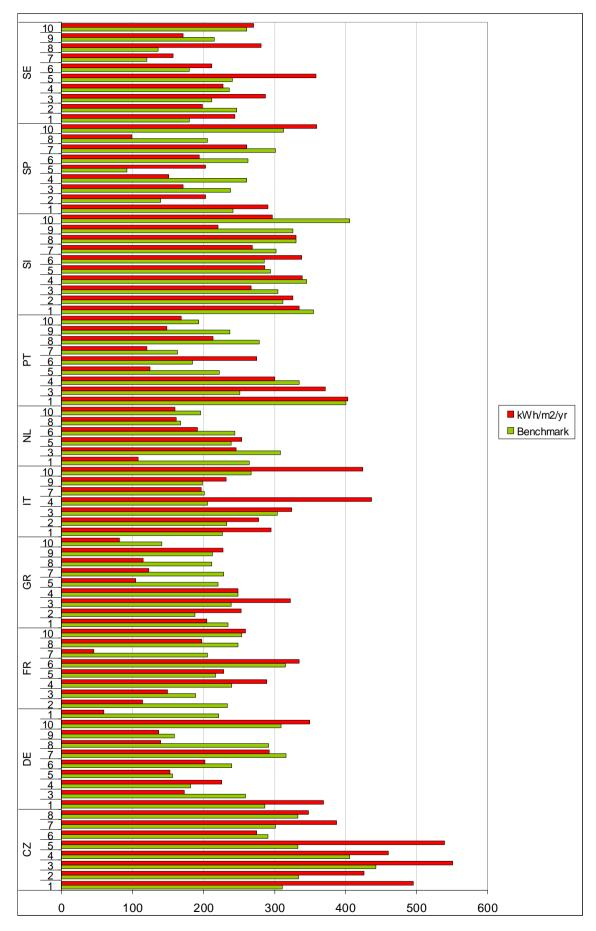
Figure 11: Real consumption per square meter, kWh/m2/yr and benchmark
