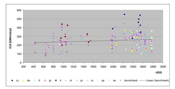
Figure 15: EUI1 (kWh all sources/m2/yr) versus HDD
