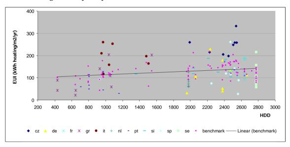
Figure 28: EUI3 (kWh heating /m2/yr) versus HDD
